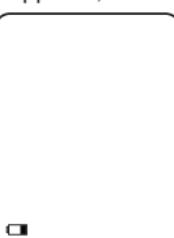
appears on the display, the batteries are almost flat and must be replaced. And after battery warning
